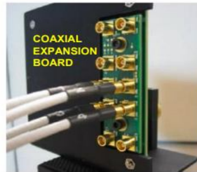
Figure 2 Transmitter Baseband Inputs
